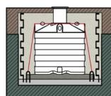
2-6mm washed gravel or Cement-stabilized sand (mixture of concrete sand and about 10% to 15% of cement)
